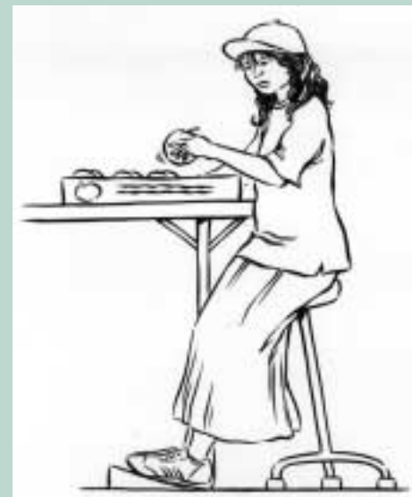
Figure 22: Proper design of workstations, including the provision of seating that allows a choice of sitting and standing, will reduce the risk of back problems.
