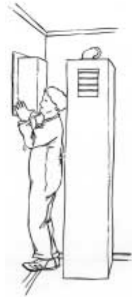
Figure 2: Poor design of equipment and facilities can create awkward manual handling tasks.
