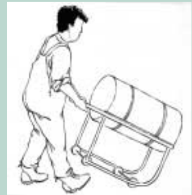
Figure 24: Drum handlers are available for most sizes of drums. This allows their convenient tilting and lifting.
