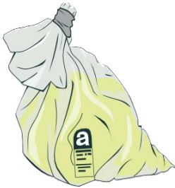
Figure 12: Double-bagged waste with 'gooseneck twist' and tape seal
