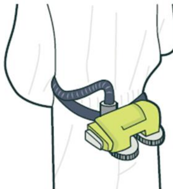
Figure 8: Common types of respiratory protective equipment (RPE) – a positive pressure respirator (suitable for stubble and beards)
