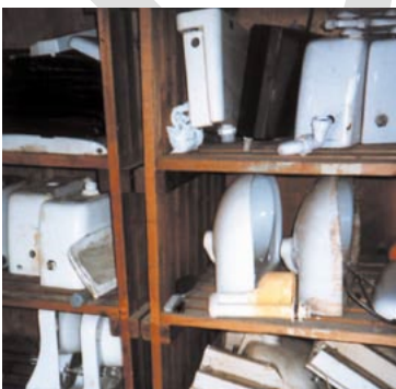
Asbestos-reinforced toilet cistern
