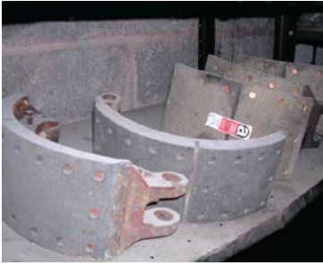
Asbestos brake linings for quarry vehicles
