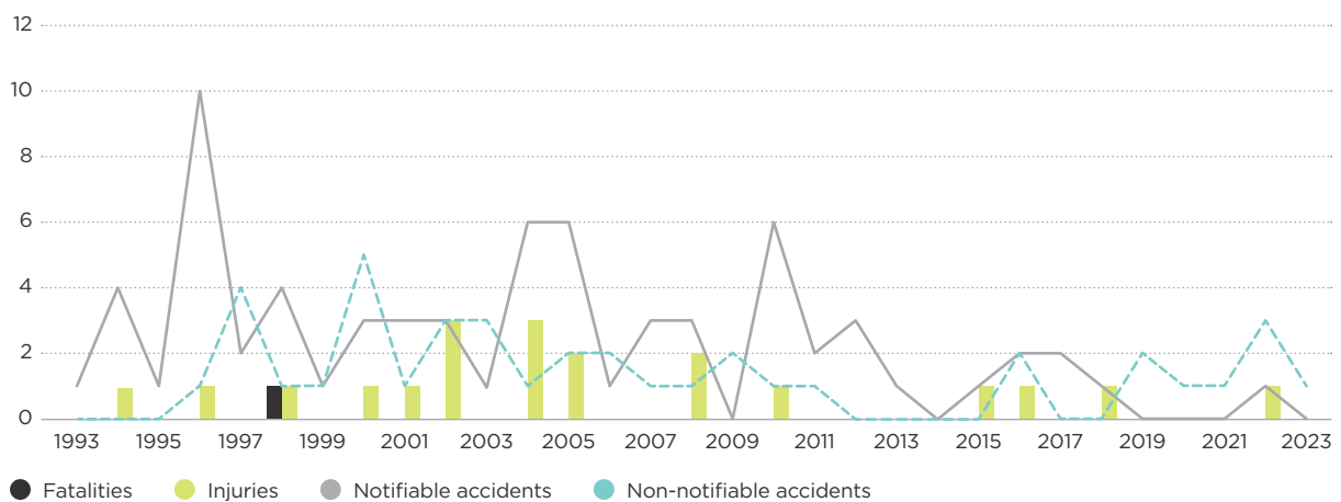
FIGURE 2I: Natural gas water heater and boiler accidents
