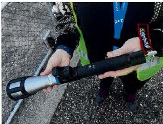
Figure 9: The new Bird Deterrent Laser ('The Bird Eraser Laser') at Auckland Airport
