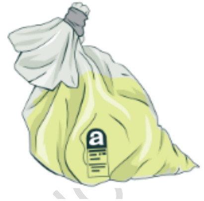
Figure 12: Asbestos waste bag tied with a gooseneck twist.
