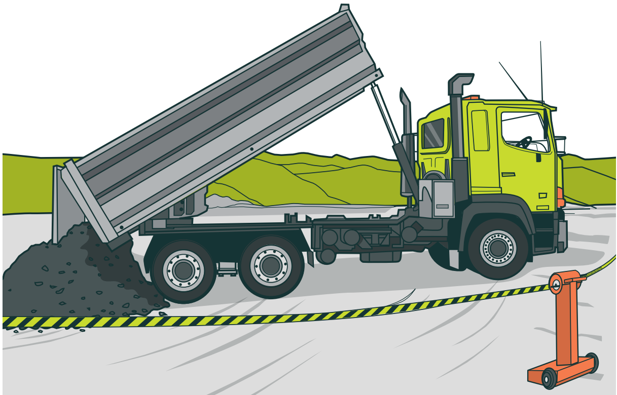
FIGURE 4: Example of a temporary barrier used to create an exclusion zone
