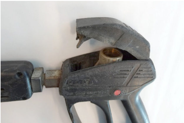
FIGURE 2: Example showing the internal structure of a solid manifold gun (gun without a bung) and trigger assembly
