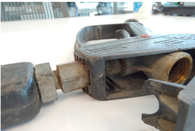
FIGURE 1: The water blaster gun involved in the incident, including the bung and threaded brass body of the gun
