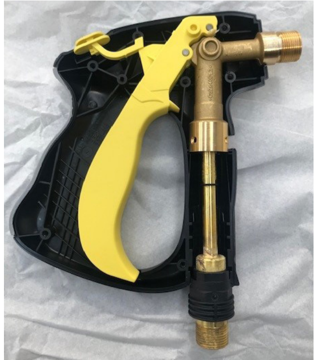
FIGURE 2: Example showing the internal structure of a solid manifold gun (gun without a bung) and trigger assembly
