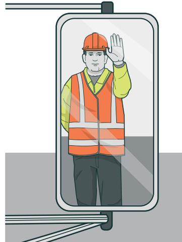
**FIGURE 9:** The view the driver should have of the spotter
