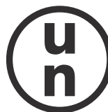
FIGURE 1: UN marking on a gas cylinder
