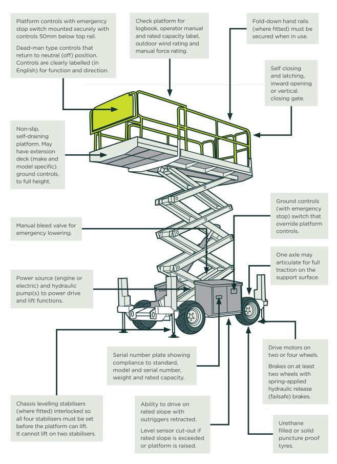
Figure 5: Typical features of scissor-lifts.
