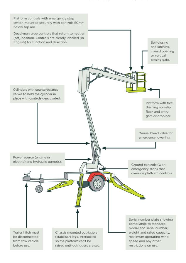
Figure 6: Typical features of trailer mounted boom-lift.
