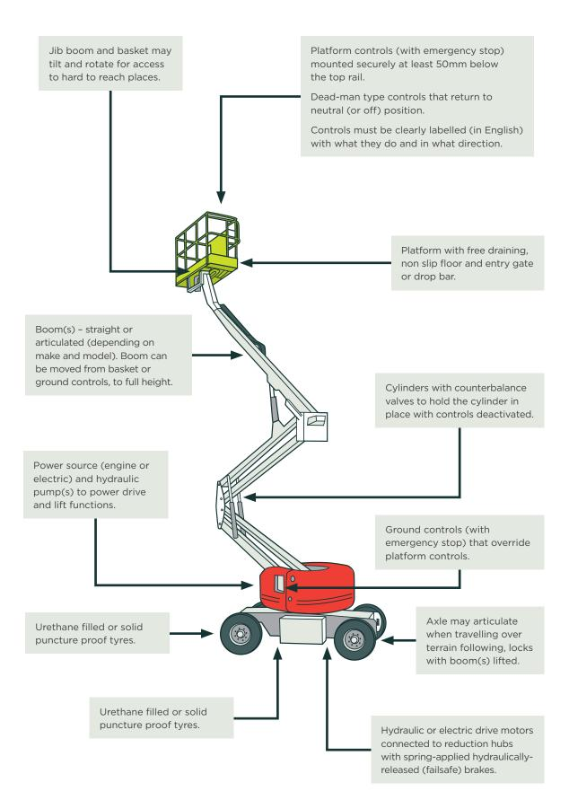
Figure 4: Typical features of self-propelled boom lifts.
