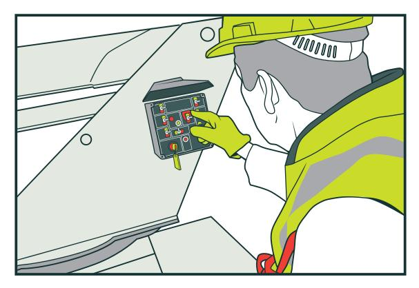
Figure 7: The operator checks the MEWP's controls before starting work.
