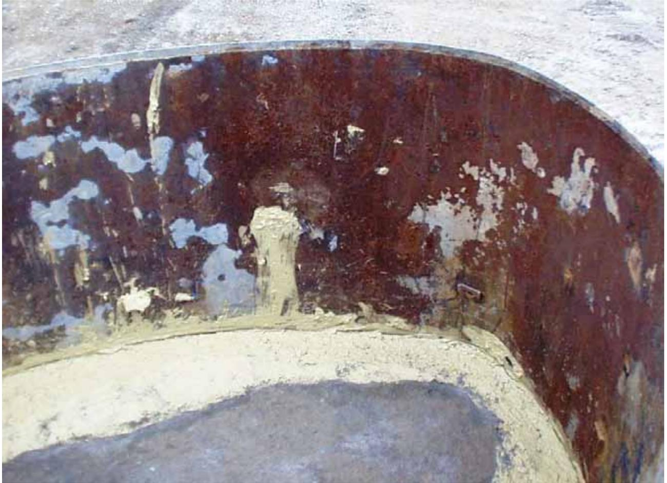
This was a simple “material at hand” existing brown rock compound floor test to gain knowledge of the suitability of the locally sourced material. The test tank was steel plate from a Tank floor replacement. It was simply made into a rough cylinder on site then welded.
