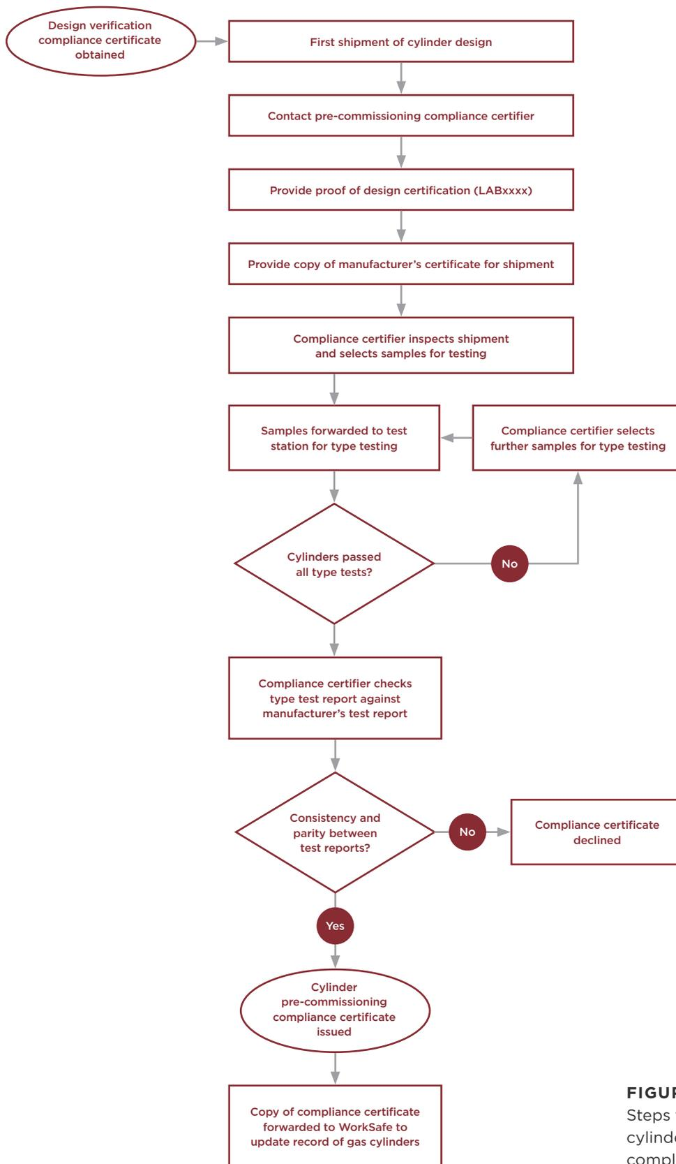
**FIGURE 2:** Steps for obtaining a cylinder pre-commissioning compliance certificate
