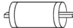
Knife-blade fuse Rarely found in domestic installations. If used, it would be for the main fuse.
