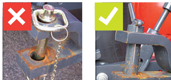
Figure 4: Correct and incorrect hitching pins
